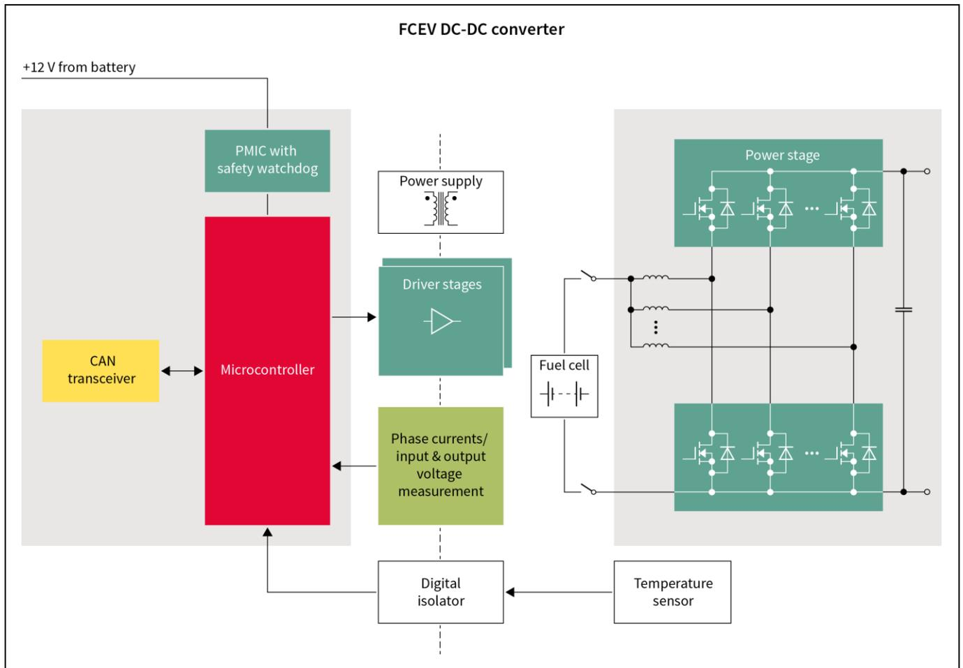
**Figure 4** The DC-DC converter produces the DC link voltage from the fuel cell stack voltage
